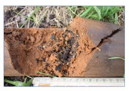
Plate 7: TP22 Probable wind blown sand at 2.5m below ground level
