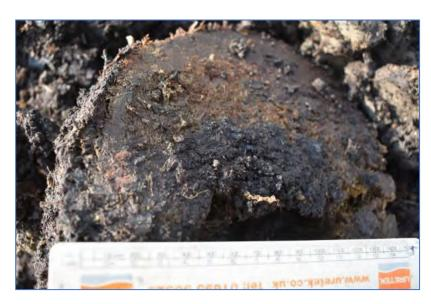
Plate 5: MW0 Fibrous peat at base of core at 1m below ground level
