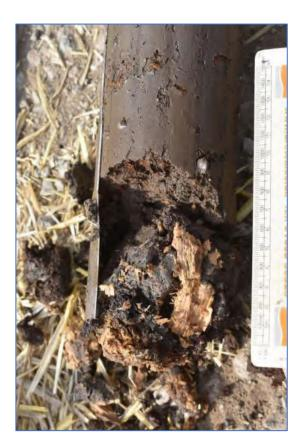
Plate 6: MW0 Fibrous and woody peat at 3m below ground level
