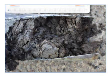
Plate 4: TP26 peat at base of core at 5m below ground level
